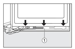
Remove panel ① from the soft-close mechanism by inserting a flat-bladed screwdriver into the gap from above and easing it off bit by bit. Take care not to damage the door seal.
